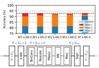
Figure 1. **Top:** Test accuracy of different binarization schemes at all stages of our cascaded distillation protocol (baseline: 92.89%). **Bottom:** The "BF2" variant of our XorEdgeConv operator.
