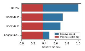
Figure 4. Relative run time on a Raspberry Pi 4B compared to the base DGCNN model. A 2x speedup is achieved by our final optimized model. Run times computed with the LCE benchmark tool over 50 runs.
