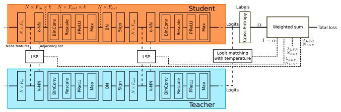
Figure 2. **Distillation with the "BF1" variant of XorEdgeConv:** the student model is more heavily quantized than the teacher. Knowledge transfer points equipped with LSP modules encourage similar dynamic graph feature distributions after each *k*-NN graph computation (except for the first, performed on the fixed 3D coordinates). Logit matching is used to further inform the training of the student.
