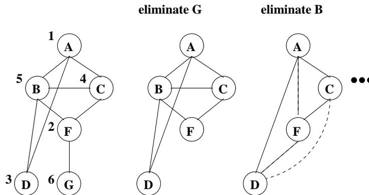
Figure B.7: Eliminating the nodes in Figure B.4, with  $\pi = (A, F, D, C, B, G)$ . Dotted edges are fill-in arcs. When we eliminate  $B$ , all the remaining nodes are lower in the ordering, and hence all neighbors of  $B$  get connected.
