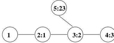
Figure B.10: Elimination tree obtained from the chordal graph of Figure B.9 using the numbering  $\{1, \dots, 5\}$ , i.e., we first eliminate 5, and ensure lower-numbered neighbors  $\{2, 3\}$  are connected, etc. From Figure 4.10 of [CDLS99].
