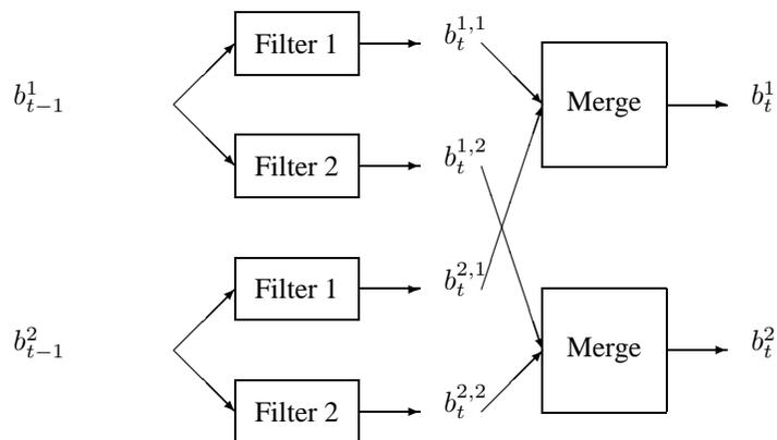
Figure 4.14: The GPB2 algorithm for the case of a binary switch.  $b_{t-1}^i = P(X_{t-1}, S_{t-1} = i | y_{1:t-1})$  is the prior,  $b_t^{i,j} = P(X_t, S_{t-1} = i, S_t = j | y_{1:t})$ , and  $b_t^j = P(X_t S_t = j | y_{1:t})$  is the approximate posterior. The filter box implements the Kalman filter equations (see Section 3.6.1). The merge box implements the weak marginalization/ moment matching equations (see Section B.5.2).
