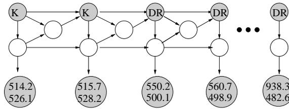
Figure 6.6: Semi-supervised training of a 2-level HHMM. The person's goal and  $(x, y)$  positions are observed, but the state,  $S_t$ , and the finished status,  $F_t$ , are hidden. K = kitchen, DR = dining room, etc.
