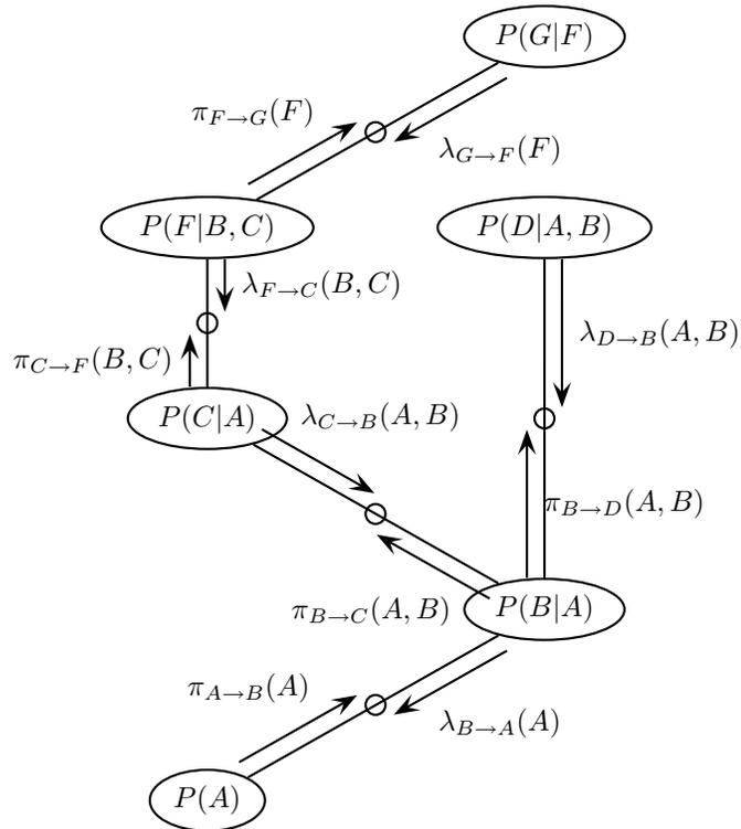
Figure B.3: The elimination tree derived from Figure B.2. Ovals represent “buckets”; the CPDs inside them are the terms they contain after initialisation. Note that the “domain” of the  $C$  bucket is  $\{A, B, C\}$ , even though it is initialized with  $P(C|A)$ . The empty circles represent separators.  $\lambda$  messages flow from the leaves to the root (the  $A$  node); then  $\pi$  messages flow from the root to the leaves.
