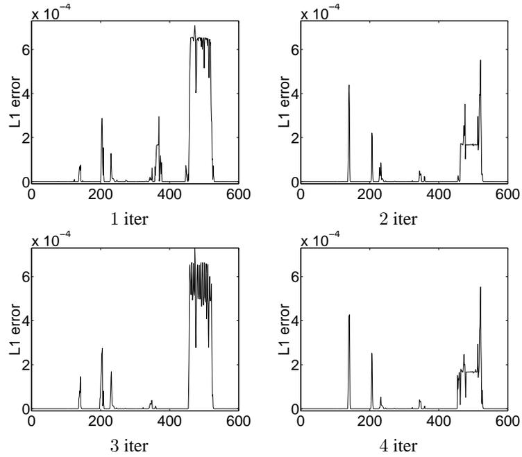
Figure 4.7:  $L_1$  error on marginal posteriors vs. timeslice after iterations 1–4 of undamped LBP applied to the traffic CHMM. The  $L_1$  error oscillates with a period of 2 (as seen by the similarity between the graphs for iterations 1/3 and 2/4); this implies that the underlying marginals are oscillating with the same period.
