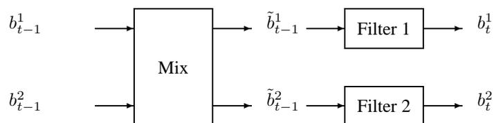
Figure 4.15: The IMM (interacting multiple models) algorithm for the case of a binary switch.
