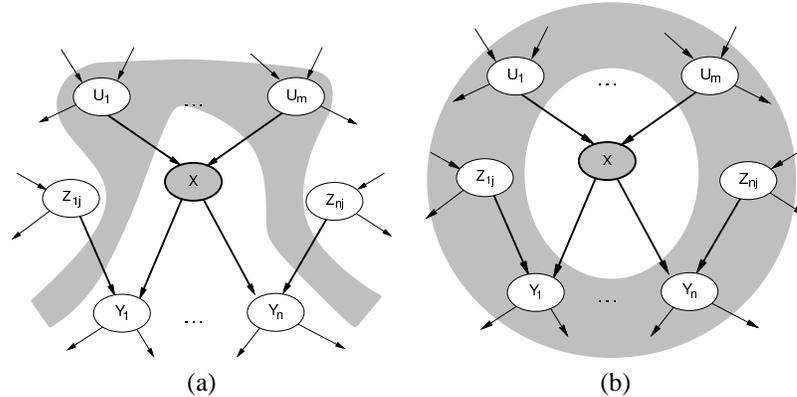
Figure A.6: Local Markov properties for Bayes nets. (a) A node  $X$  is conditionally independent of its non-descendants (e.g.,  $Z_{1j}, \dots, Z_{nj}$ ) given its parents  $U_1, \dots, U_m$ . (b) A node  $X$  is conditionally independent of all other nodes in the network given its Markov blanket (shaded). From [RN02].
