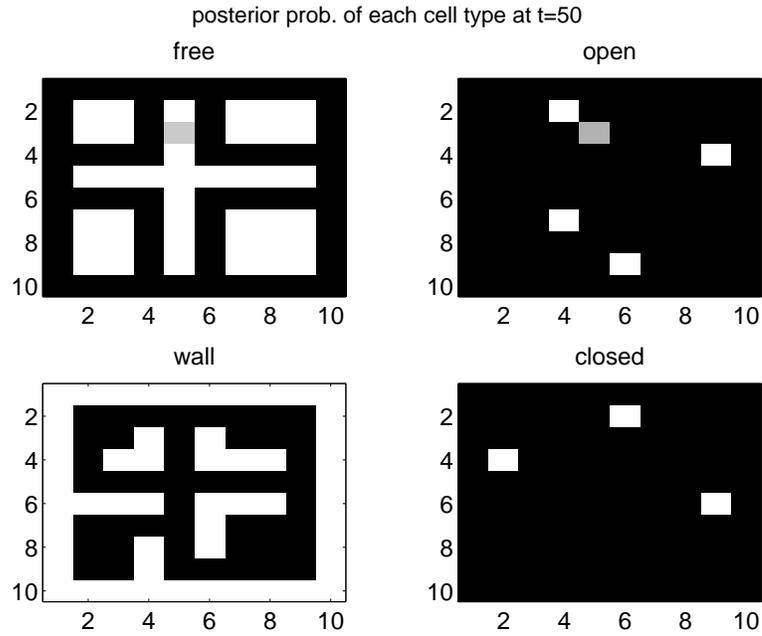
Figure 5.13: Results of RBPF on the 2D grid world using 200 particles. Cell  $(i, j)$  in the top left figure represents  $P(M_t(i, j) = \text{free} | z_{1:t})$  using a gray scale, and similarly for the other three figures. Hence the open doors correspond to white blobs on the top right figure, etc.
