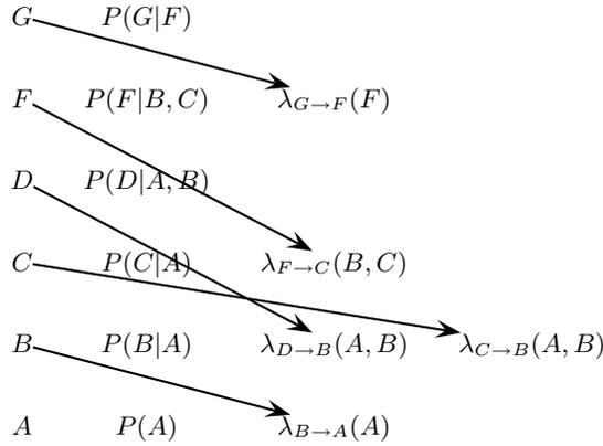
Figure B.2: Variable elimination applied to Figure B.1 using the ordering  $A, B, C, D, F, G$ . The arrow from  $F$  to  $C$  means we compute the “message”  $\lambda_{F \rightarrow C}(B, C) = \sum_F P(F|C, B)\lambda_{G \rightarrow F}(F)$  and send it to  $C$ ’s “bucket”, etc.
