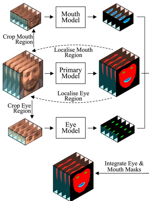
**Fig. 2** An illustration of how the primary and zoomed-in models work. The primary face masks are extracted out of the video sequence by the primary model, and these masks are used to localise the mouth and eye regions. The cropped mouth and eye sequences are then fed into the additional mouth and eye models, respectively, to extract mouth and eye masks at higher accuracies. The primary face mask, eye and mouth masks are then combined to obtain the final face mask. (Best seen in colour)
