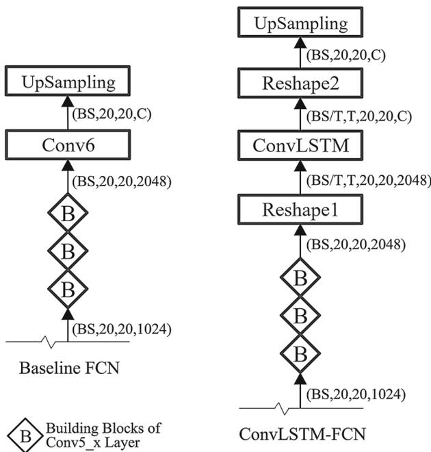
**Fig. 1** An illustration of casting baseline FCN into ConvLSTM-FCN model. Only these top layers are shown. ‘BS’ refers to batch size of images, ‘T’ denotes the time dimension in ConvLSTM layer and ‘C’ is the target classes number. The ConvLSTM layer in ConvLSTM-FCN has the same convolutional filters with Conv6 layer in Baseline FCN. Two reshape layers are added to convert tensor dimensions in ConvLSTM-FCN
